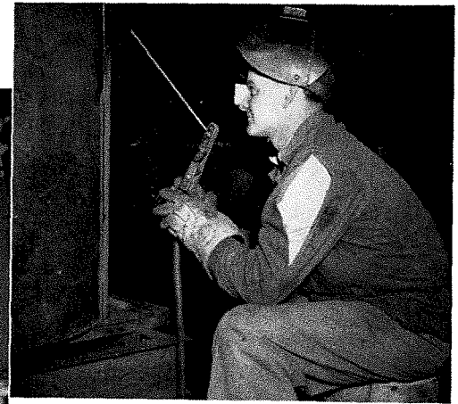
DENVER JOHNSON seam welding an abrasive separator.
