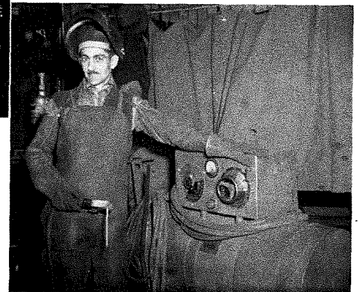
LESTER NEDDEAU standing beside one of the modern welding units used in our factory, demonstrates the protective clothing worn by welders — leather apron, arm shields, gloves and helmet.
